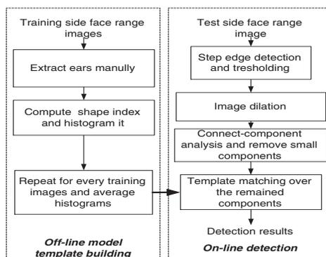
Figure 1. System diagram.
